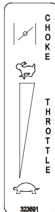
15 HP Kawasaki Units Engine Code FH451V-AS04 PART NO. 1-323691 LOCATION: RH Side of Console
